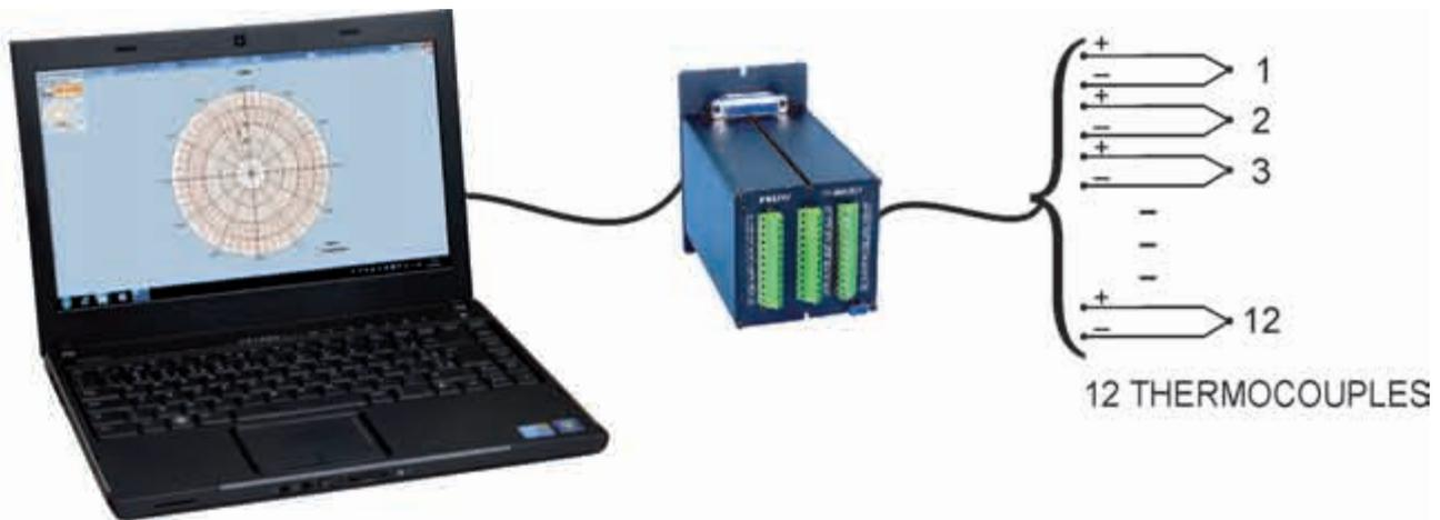
Example of VR-2000 use with the TY-2095 measuring 12 temperature points from thermocouple inputs. It can simulate 12 records of a pen each or 6 records of two pens, or any desired combination.
