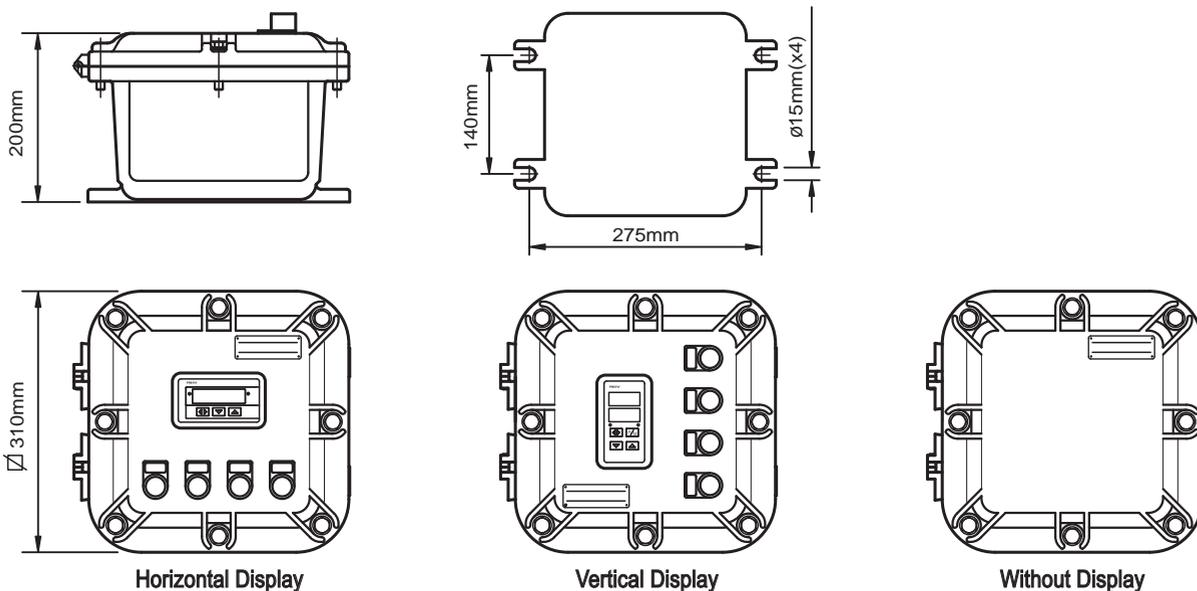
NOTE: Command buttons with mounting option for 1, 2, 3, 4 buttons or none.
